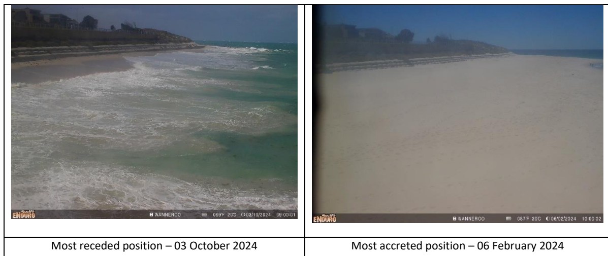
Figure 6-3 Most receded and most accreted shoreline positions to the south of Quinns Rocks Groyne One (1) during the study period.
