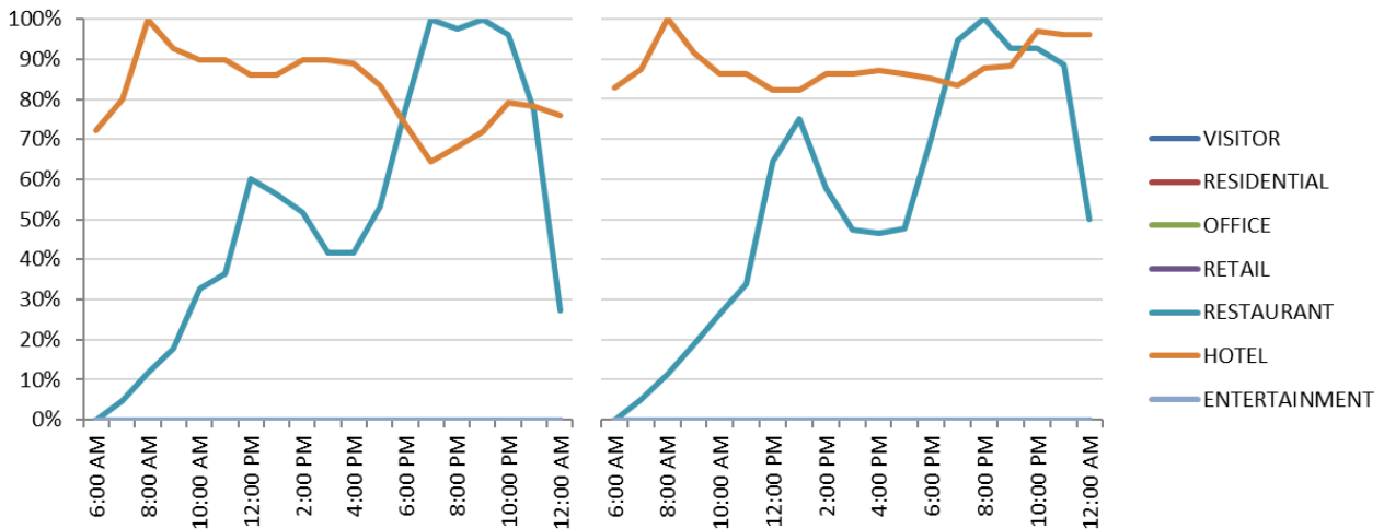
Figure 3.11 Development land use parking profiles by category – weekdays (left) and weekends (right)
