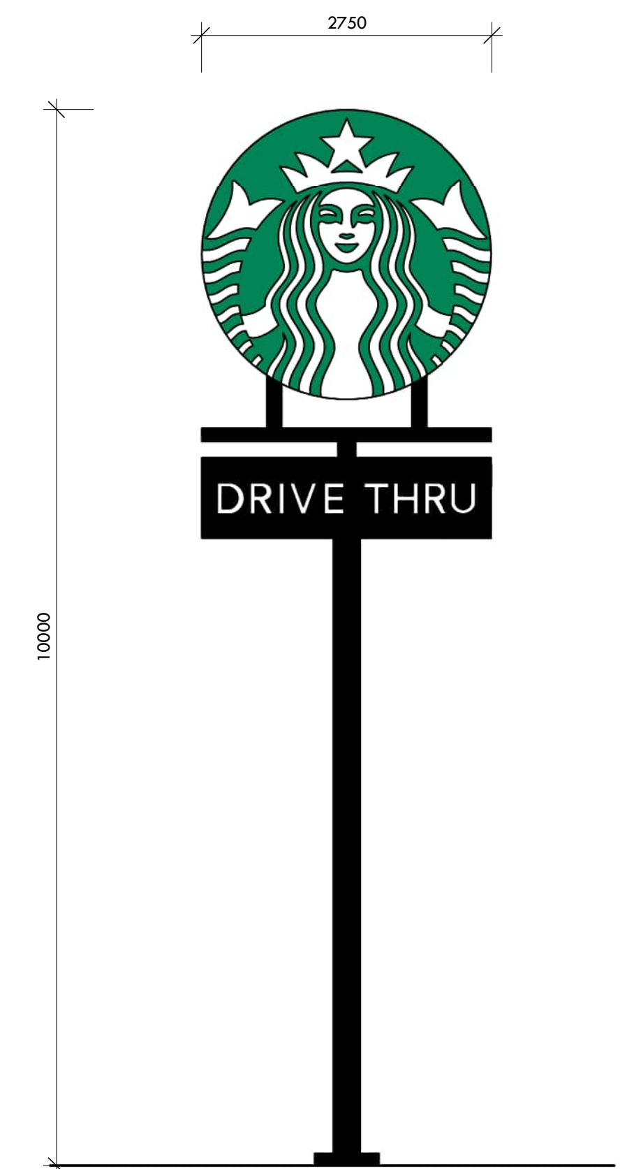
PYLON SIGN ELEVATION
