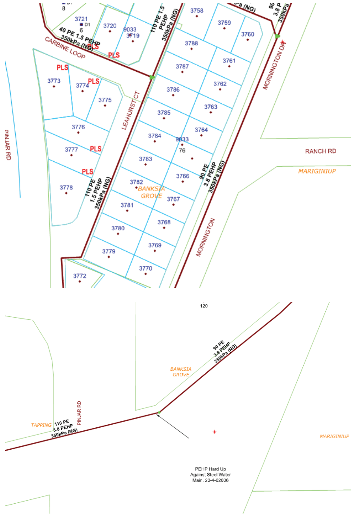
Figure 9: Existing Gas Infrastructure
